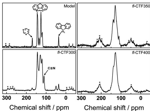
Fig. 2  $^{13}\text{C}$  MAS ssNMR spectra of tris(9*H*-fluorene-2-yl)-1,3,5-triazine (top left), *fl*-CTF300 (bottom left), *fl*-CTF350 (top right) and *fl*-CTF400 (bottom left). Asterisks mark rotational side bands.
