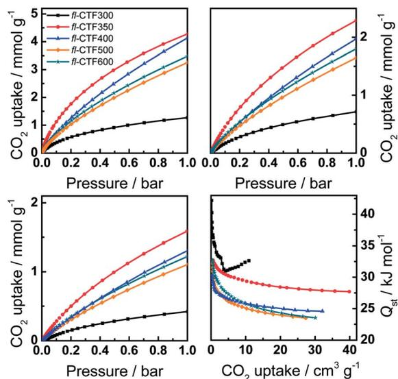
Fig. 5 Carbon dioxide adsorption isotherms of *fl*-CTF300, *fl*-CTF350, *fl*-CTF400, *fl*-CTF500 and *fl*-CTF600 at 273 K (top left), 298 K (top right), 313 K (bottom left) and corresponding heats of adsorption (bottom right).
