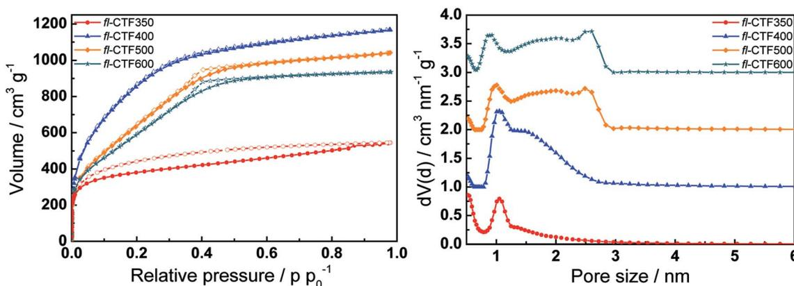
Fig. 3 (Left) Argon adsorption (filled symbols) and desorption (open symbols) isotherms at 87 K of *fl*-CTF350, *fl*-CTF400, *fl*-CTF500 and *fl*-CTF600. (Right) Pore size distributions of *fl*-CTF350, *fl*-CTF400, *fl*-CTF500 and *fl*-CTF600 from DFT calculations. The curves are shifted vertically in steps of 1  $\text{cm}^3 \text{nm}^{-1} \text{g}^{-1}$ .
